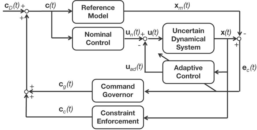
**Fig. 1** Block diagram of overall control structure
