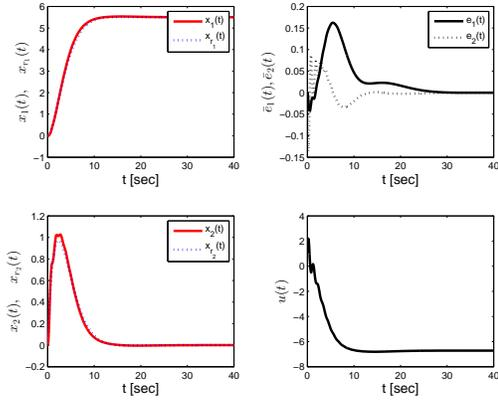
Fig. 5. System response and tracking error with command governor rate  $\lambda = 15$  and input filter  $\mathcal{G}_{u \rightarrow u_f}(s)u(s) = \frac{25}{s+25}$  for a unity step command.
