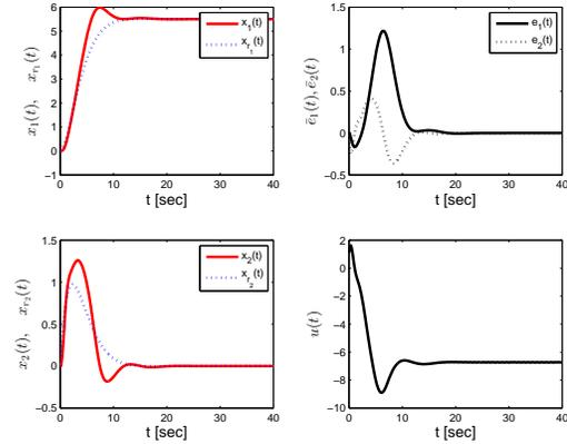
Fig. 6. System response and tracking error with command governor rate  $\lambda = 15$  and input filter  $\mathcal{G}_{u \rightarrow u_f}(s)u(s) = \frac{5}{s+5}$  for a unity step command.
