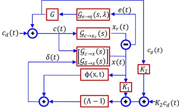
Fig. 1. Augmented System Represented as Interconnected Transfer Functions Blocks
