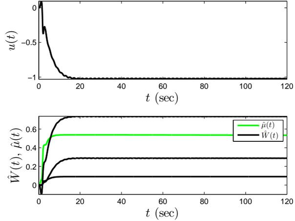
Fig. 4. Control signal and weight update law responses for the proposed model reference adaptive controller in Theorem 2.
