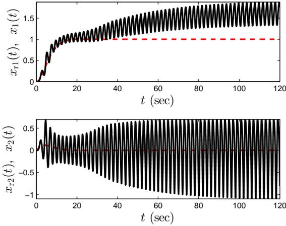
Fig. 1. System state and reference state responses for the standard model reference adaptive controller in Theorem 1.
