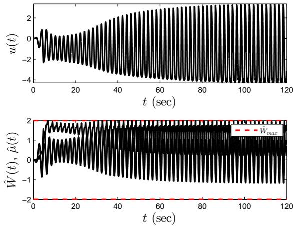
Fig. 2. Control signal and weight update law responses for the standard model reference adaptive controller in Theorem 1.
